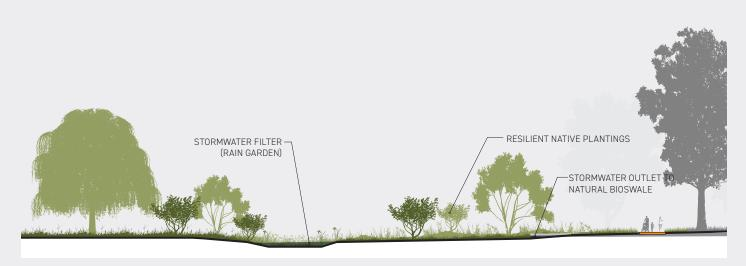
SECTION THROUGH STORMWATER DAYLIGHTING
