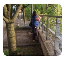
**DO NOT DO THIS** Railing height should be 42", typ. from ground plane wherever feasible throughout the corridor to allow for unobstructed views of the river and fishing access.
